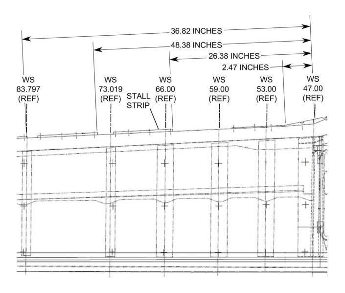
Figure 1. Bonanza Stall Strip Relocation (Sheet 3)
