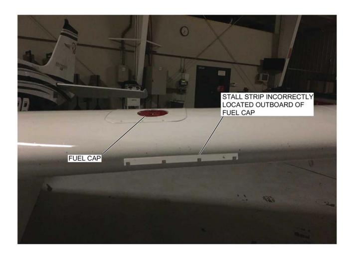
Figure 1. Bonanza Stall Strip Relocation (Sheet 1)
