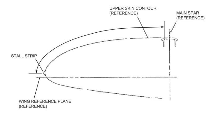
Figure 1. Bonanza Stall Strip Relocation (Sheet 4)
