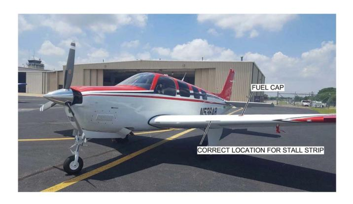
Figure 1. Bonanza Stall Strip Relocation (Sheet 2)
