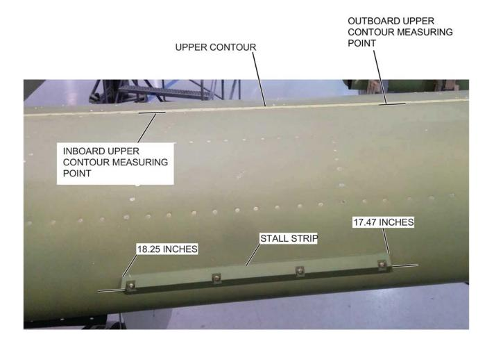
Figure 1. Bonanza Stall Strip Relocation (Sheet 5)
